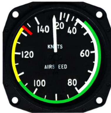
Figure 2.1.1 Analog Airspeed Indicator Marks
