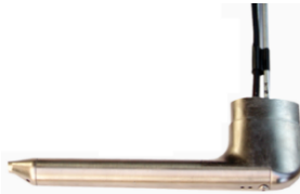
Figure 7.7.1 Pitot Tube Probe
